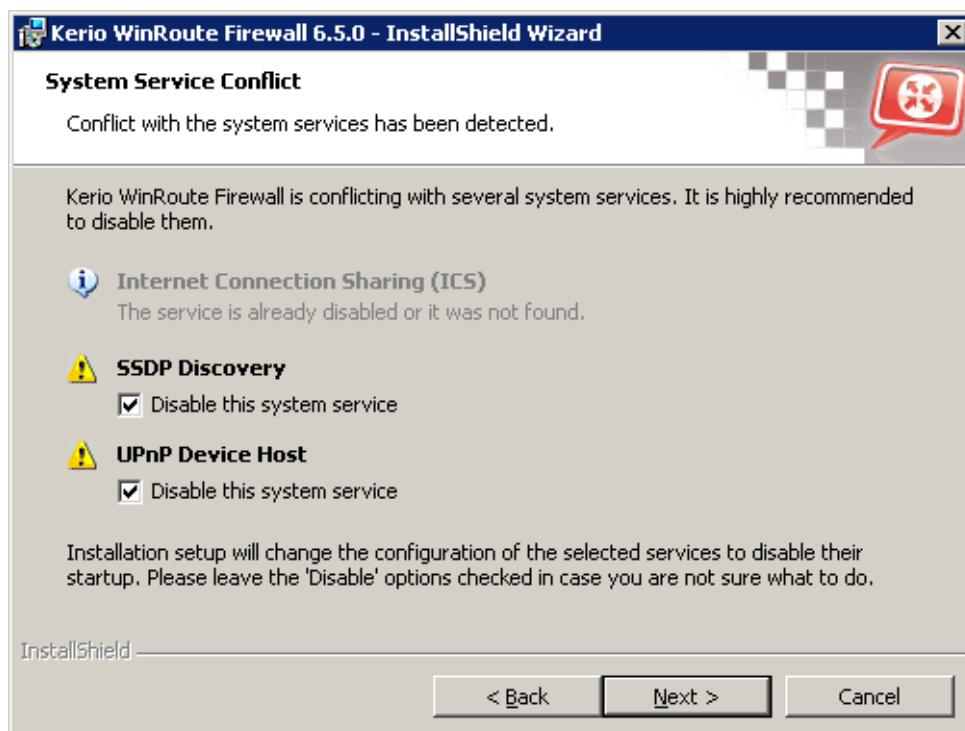
Figure 2.2 Disabling colliding system services during installation
