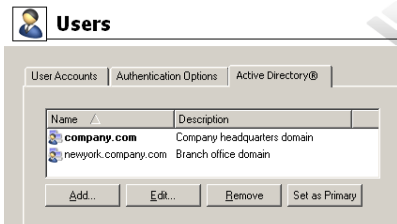
Figure 15.15 Mapping of multiple Active Directory domains
