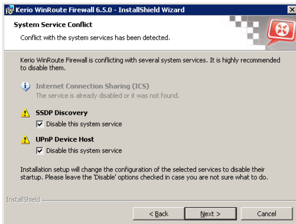
Figure 2.2 Disabling colliding system services during installation
